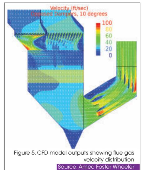
Figure 5. CFD model outputs showing flue gas velocity distribution
