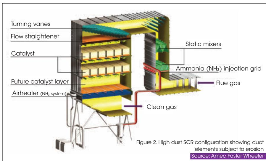
Figure 2. High dust SCR configuration showing duct elements subject to erosion
