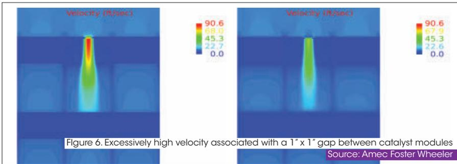
Figure 6. Excessively high velocity associated with a 1" x 1" gap between catalyst modules
