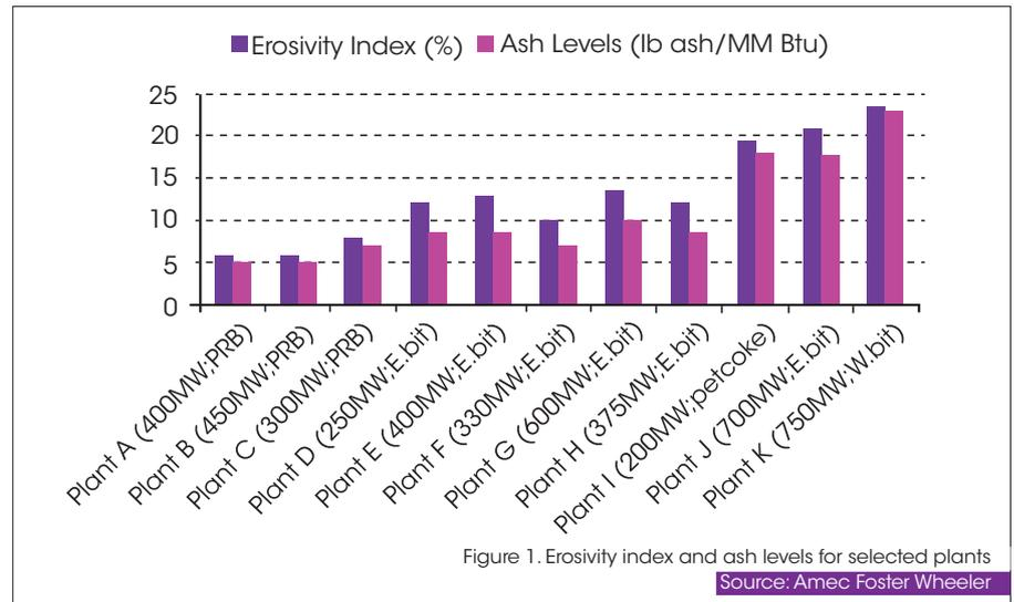
Figure 1. Erosivity index and ash levels for selected plants
